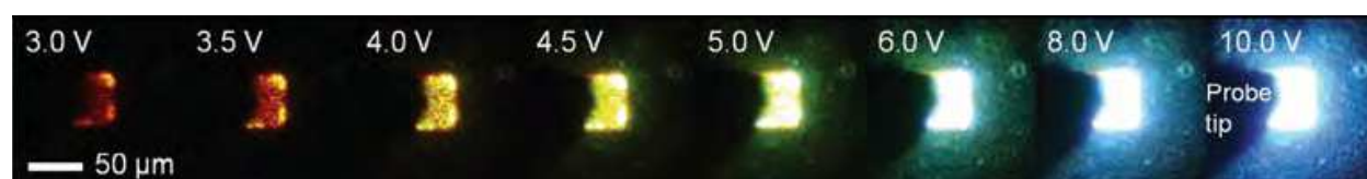
Fig. 12. Color tunability varying the voltage in a PFO-QD (70-30) based emissive film. Source: (Hong et al., 2011).
