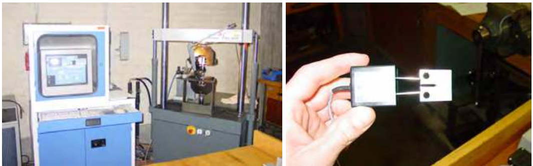
Fig. 9. Experimental tests for determining of J values
