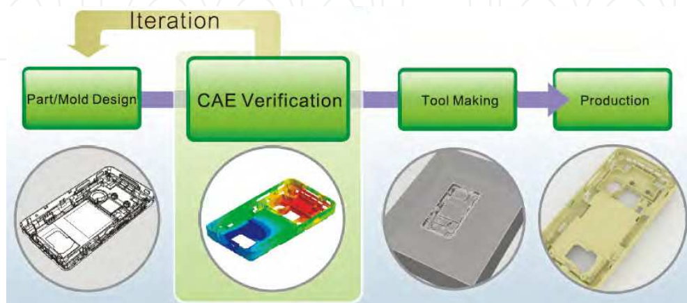
Fig. 8. Mold design process
