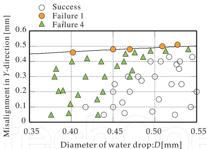
Fig. 21. Relation between the diameter of the drop and the misalignment in the Y-direction for picking up a cylindrical object.
