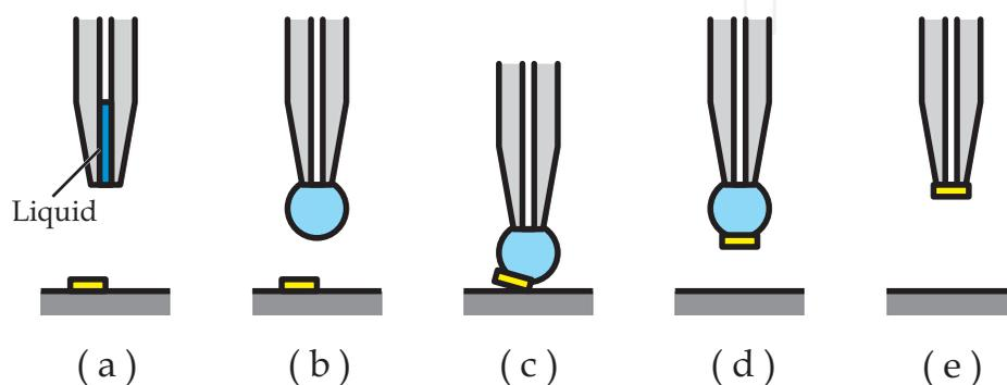
Fig. 2. Process of assembly using water drop
