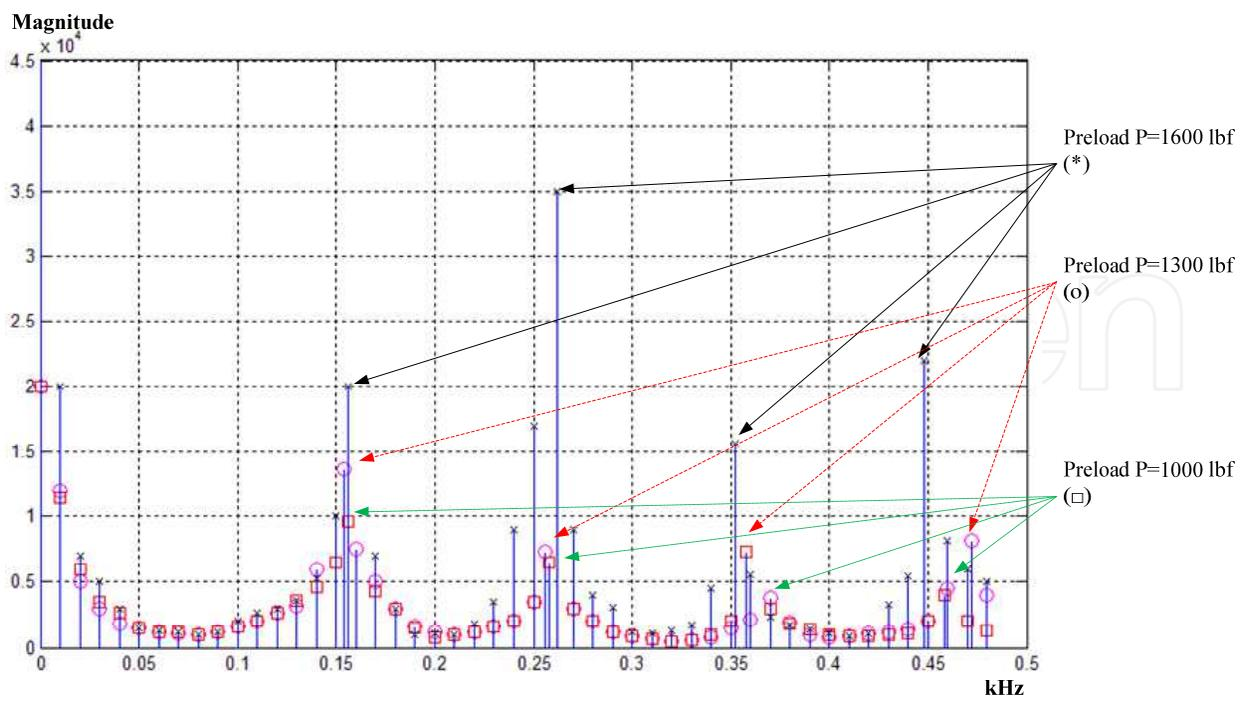
Fig. 10. A simplified illustration on the Frequency Response Functions (FRF) of the Test System
