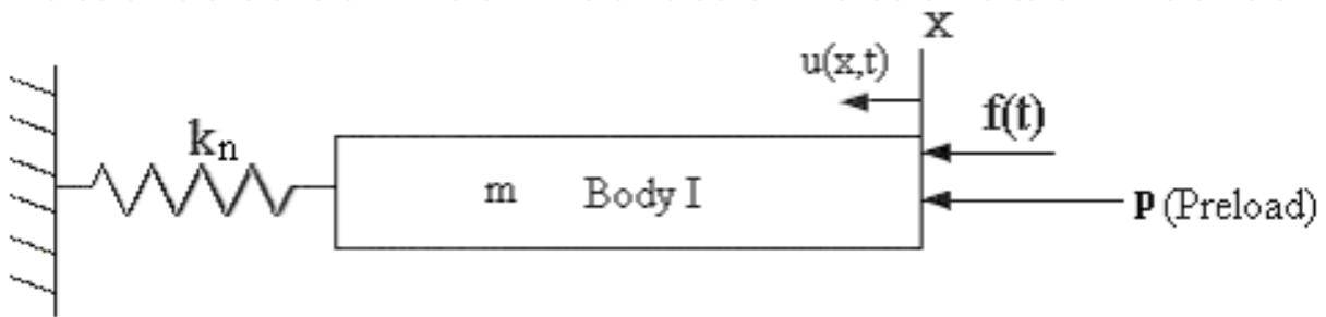
Fig. 7. One-Dimensional Model for Normal contact Stiffness
