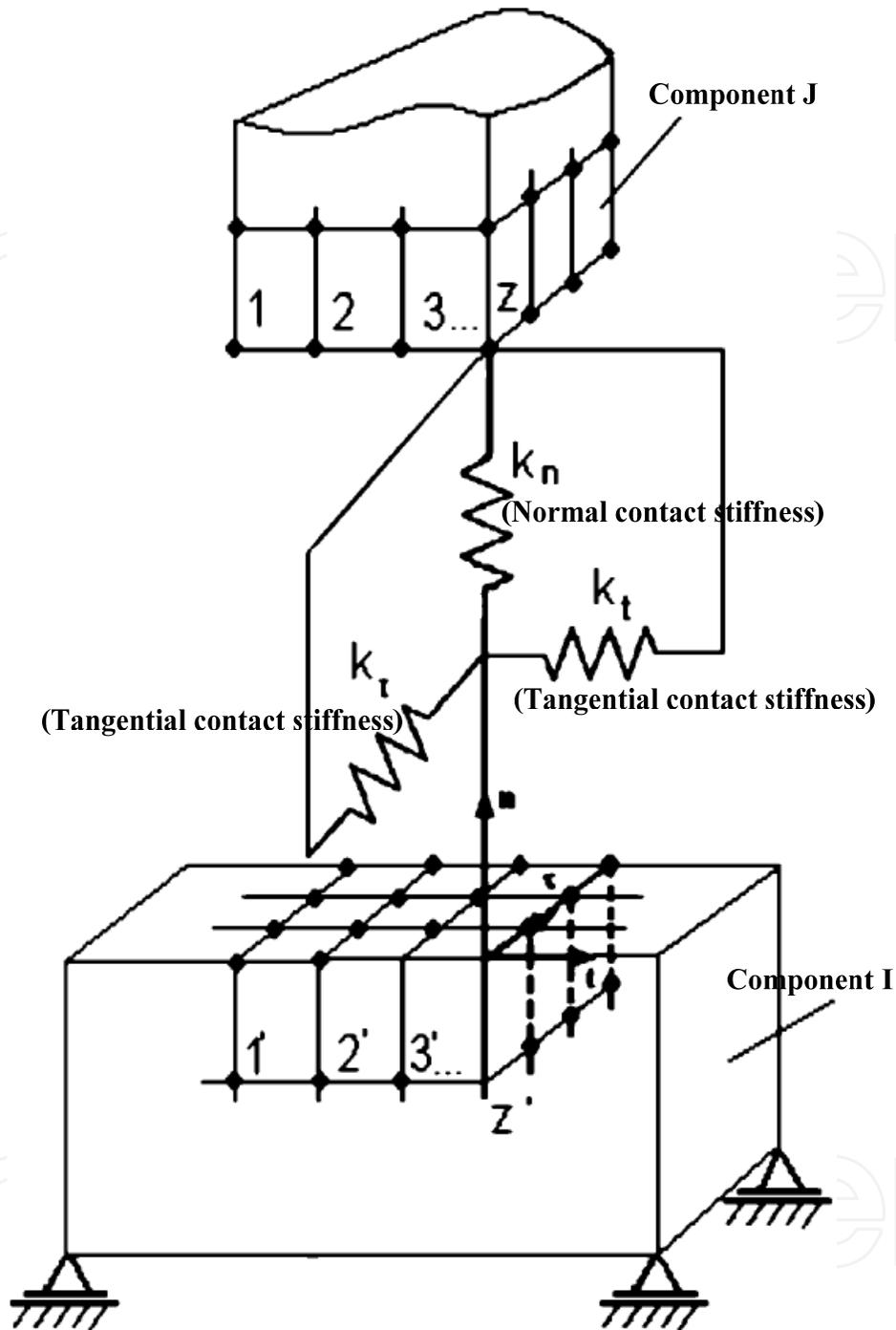
Fig. 3. Contact Model of Two Fixture Components
