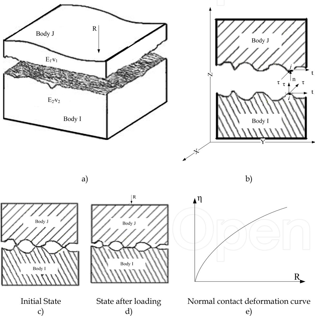
Fig. 4. Physical Model of the Contact Conditions
