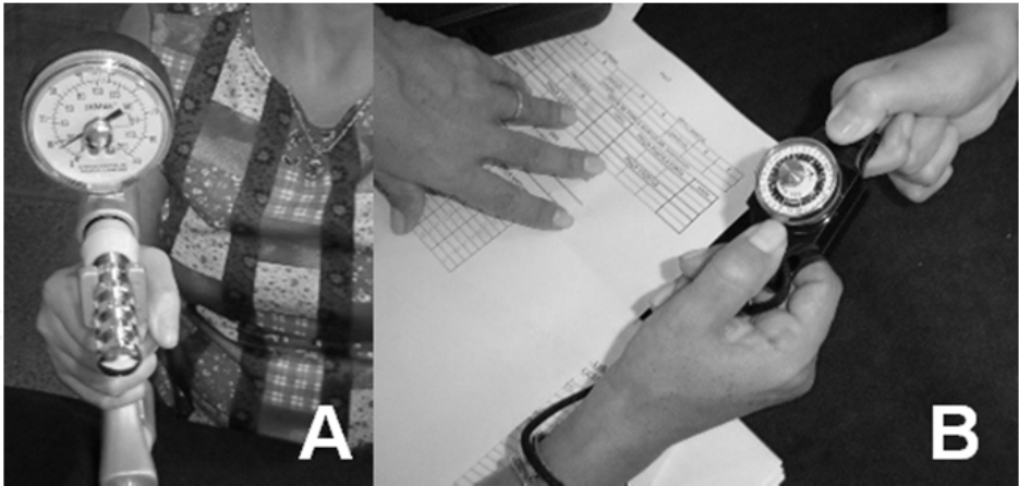
Fig. 3. The Jamar™ (A) and Pinch Gauge™ (B) dynamometers.
