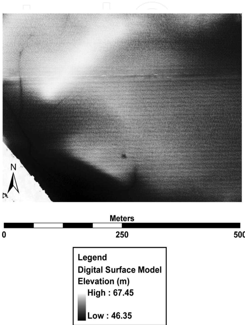
Fig. 10. Step error corrected (Willers et al., 2008a) laser scanning elevations from 2003 for the same region of the two cotton fields.
