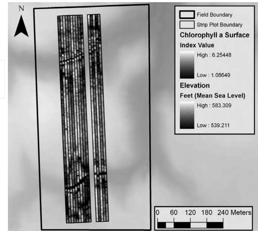
Fig. 5. Illustration of some of the geo-spatial relationships for a site-specific nitrogen experiment in a Nebraska corn field. The background is a laser scanning surface of elevational relief (Feet Mean Sea Level).
