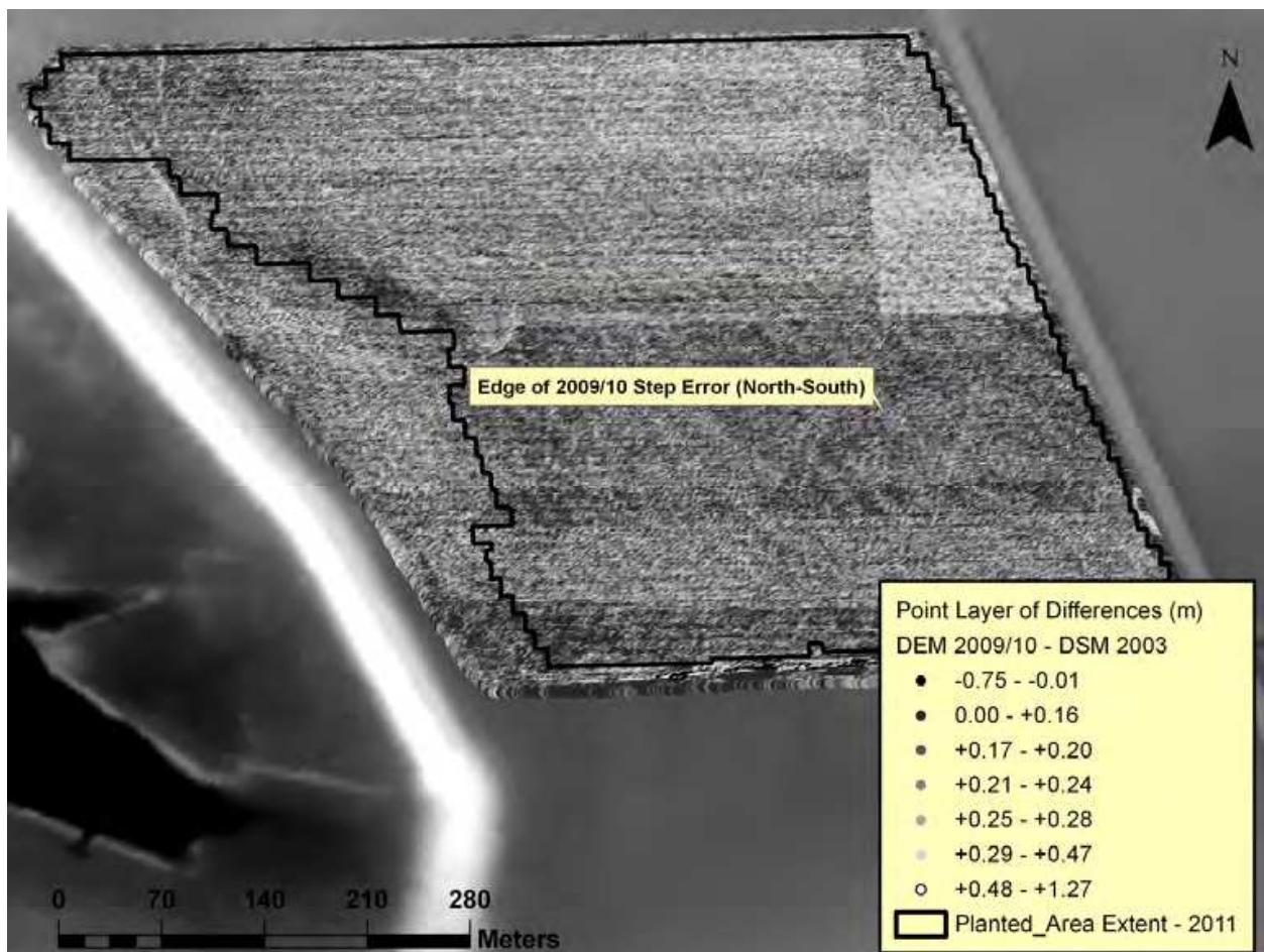
Fig. 7. Potential step error revealed by differences of the 2009/2010 bare earth DEM and the step corrected 2003 DSM.
