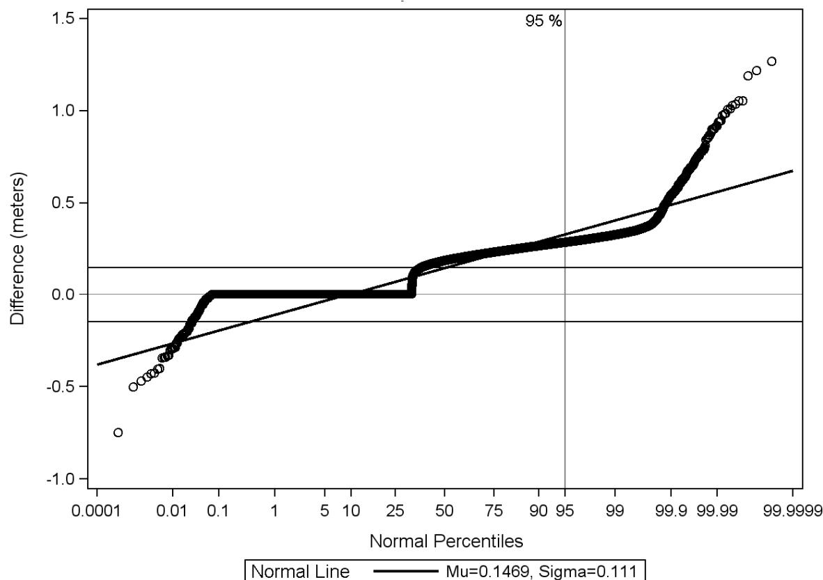
Fig. 6. Probability plot of the elevation difference between a 2009-2019 digital elevation model and a step error corrected (Willers et al., 2008a), 2003 digital elevation model.
