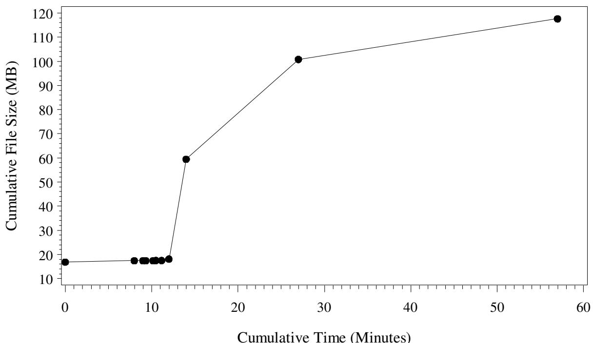
Fig. 17. Illustration of the relationship between cumulative time and cumulative file size for a task combining laser scanning elevation model with a raster layer of arctan normalized difference vegetation index values for one field on a commercial farm.
