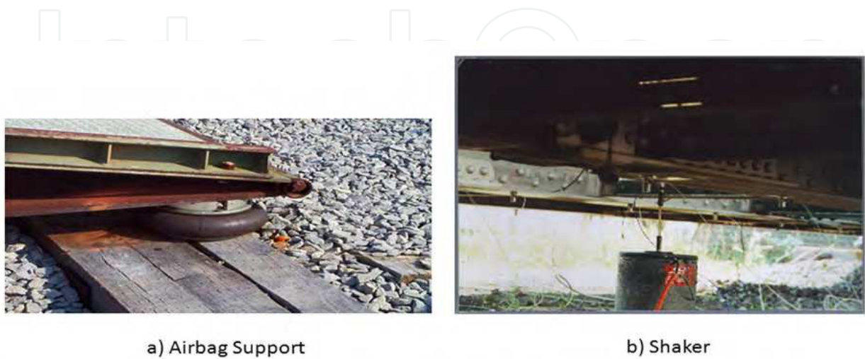
Fig. 12. Testing Setup: a) Airbag and b) Shaker
