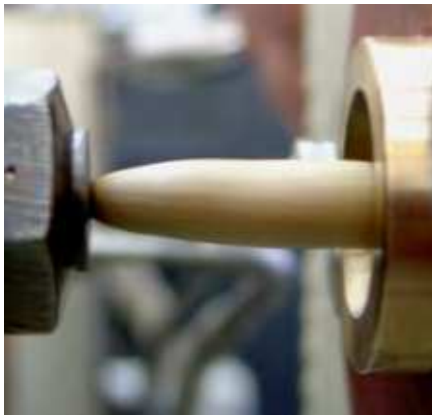
Fig. 33. Extrusion foaming of PP filled with 30 wt.% of wood flour
