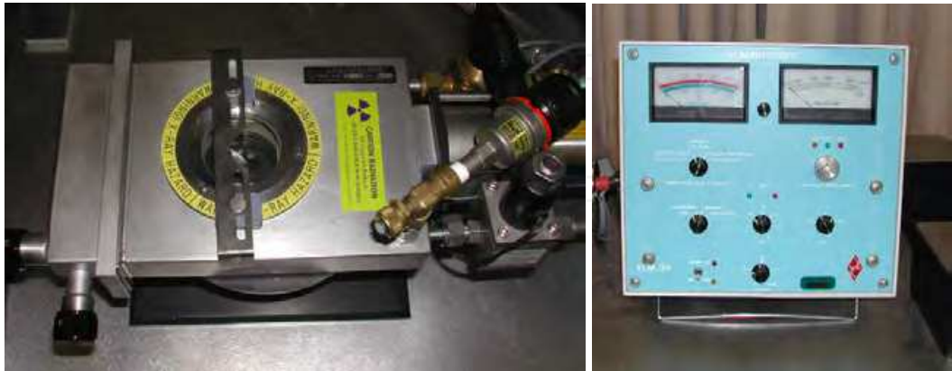
Fig. 2.4. Left: Luminoscope sample holder. Right: Luminoscope control and electronics.
