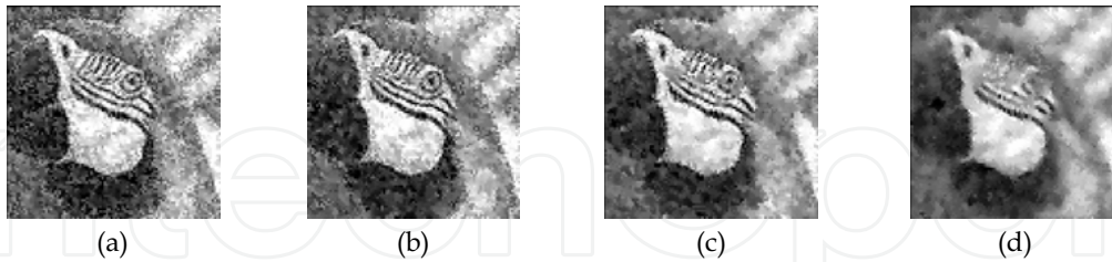
Fig. 5. Result of applying the improved filter with different \beta : (a) 50%, (b) 75%, (c) 90% and (d) 100% of the maximal value of c(x) .
