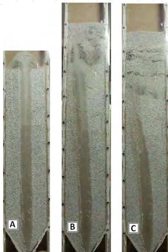
Fig. 14. Half sectional column tests at H: a) external spout and fountain formation at H \approx 0.95 H_m , b) submerged spouting at H \approx 1.05 H_m c) spouting instability with spout wandering at H \approx 1.05 H_m
