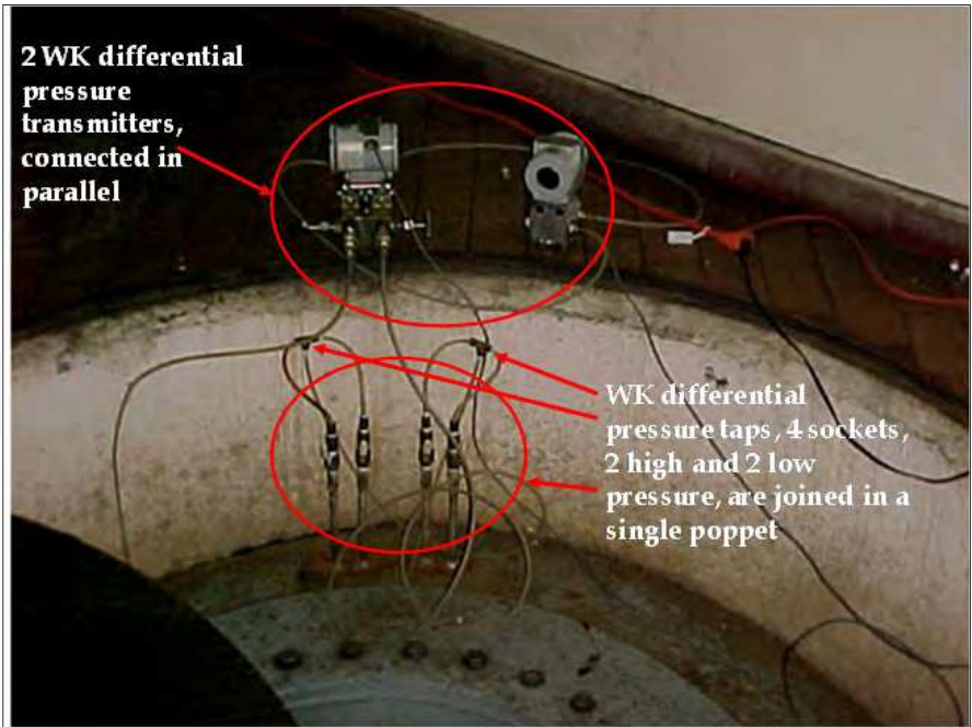
Fig. 7. Position of pressure transmitters outside of the spiral case.
