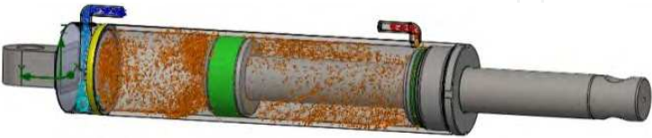
Fig. 14. Flow trajectories inside the hydraulic cylinder at L = 185 mm (see table 2).
