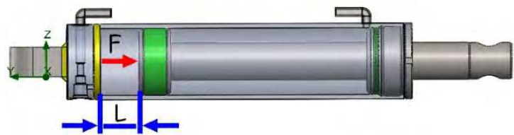
Fig. 7. Operating volume of the hydraulic cylinder
