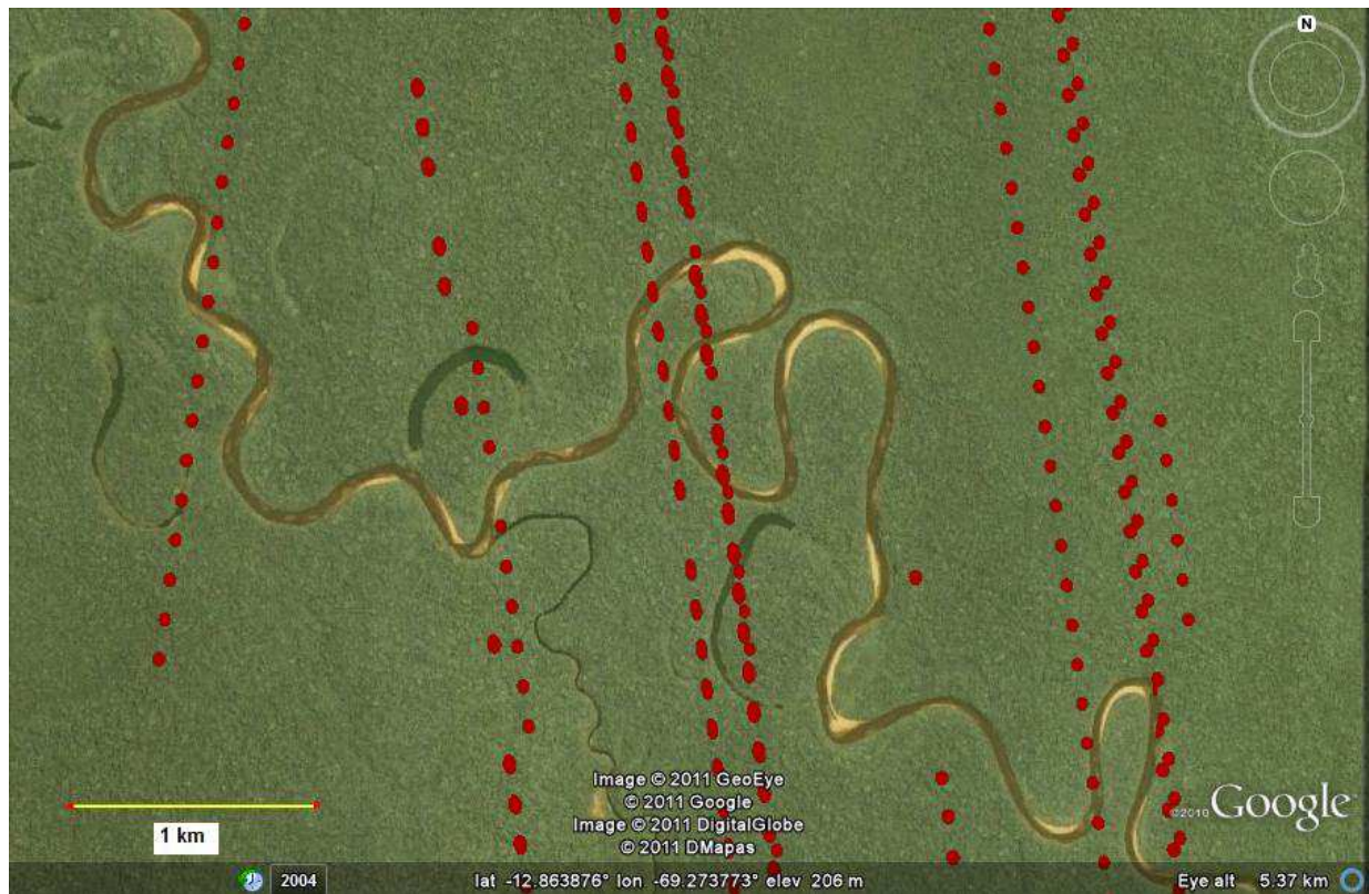
Fig. 3. Multiple GLAS laser campaigns sampling overlaid on a GoogleEarth image of Tambopata, Peru. Missing data are found where dense cloud prevents sufficient energy from penetrating to the Earth's surface and returning to the sensor.
