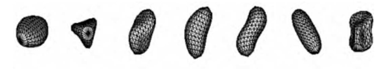
Fig. 2. Graphical representation of seven low frequencies vibration modes for surface model of ellipsoids [Syn and Prager, 1994]
