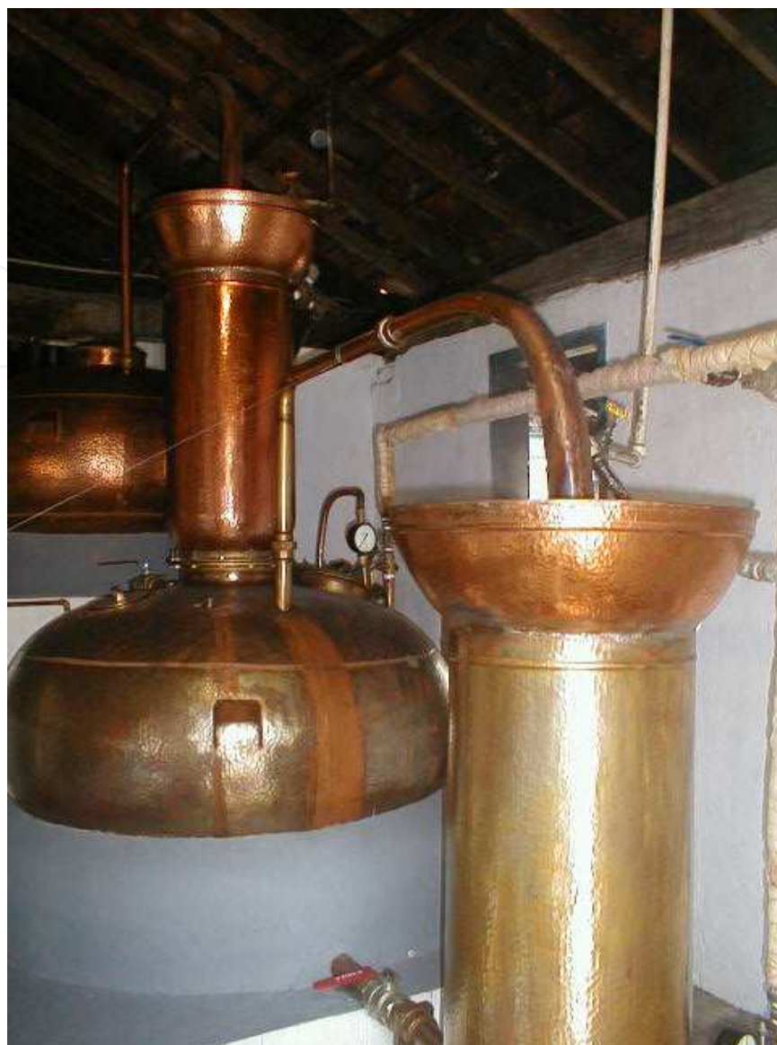
Fig. 13. Alembic of three bodies (CHV) with a hood-type cooling system (Vassouras/RJ).
