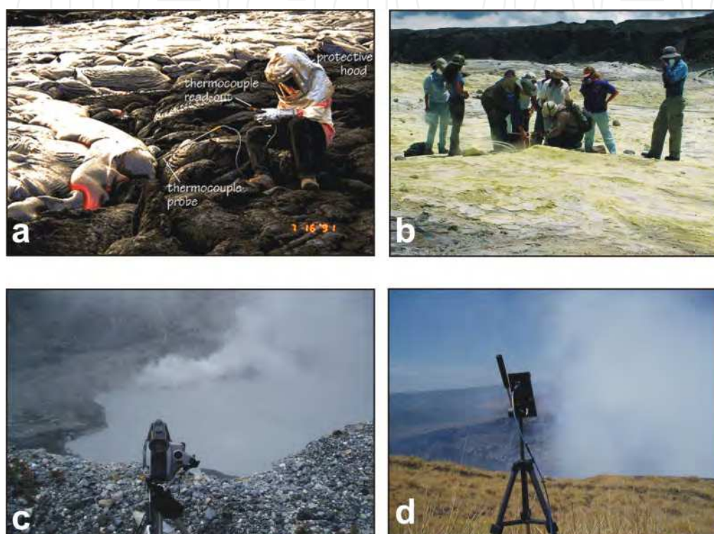
Fig. 1. Different modes for temperature and volcanic gas sampling. Conventional in situ measurements of (a) the temperature of Hawaiian pāhoehoe lava flow fields (photo by P. Mougini-Mark, volcano.oregonstate.edu), and (b) volcanic gas from the summit fumarole field of Kilauea volcano in 2005. In (c) and (d) ground-based thermal imagery of the Laguna Caliente crater lake (Poás volcano, Costa Rica; 2009) and UV-DOAS measurements of the Santiago crater (Masaya volcano, Nicaragua; 2009) volcanic plume, respectively.
