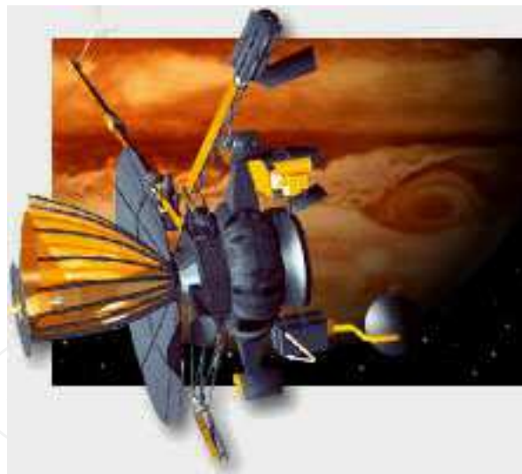
Fig. 16. Galileo's Undeployed HGA.
