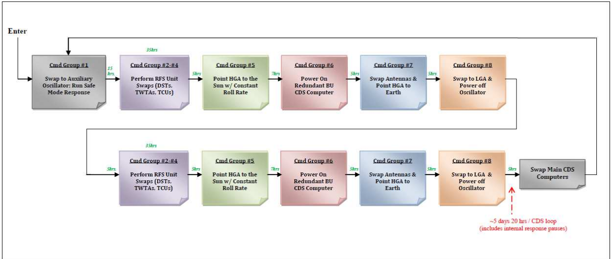
Fig. 7. Cassini’s Command Loss Response Chain for One CDS Cycle (Endless Loop Response).
