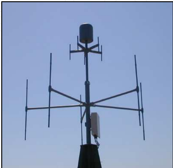
Fig. 6. Five element Uniform Circular Array interferometer
