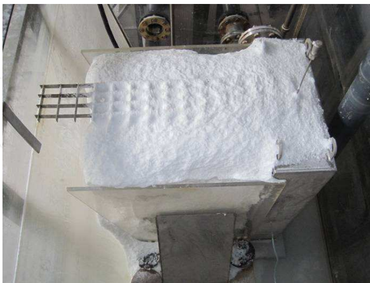
Fig. 17. Post-test photograph of full fiber/particulate load test
