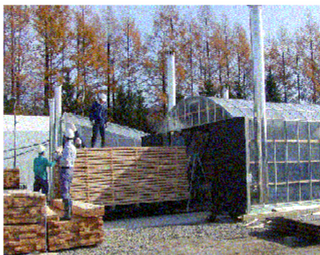
Photo 1. A Fully Passive Solar Lumber Drying House Loading Larch Lumber (2×4 material); (South-North model)
