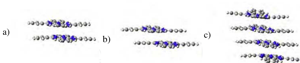
Fig. 2. DFT calculated optimized structures of H_2Pc dimers and tetramer. In the figure, a) \alpha -modification of H_2Pc dimer b) \beta -modification of H_2Pc dimer c) \alpha -modification of H_2Pc tetramer, respectively.
