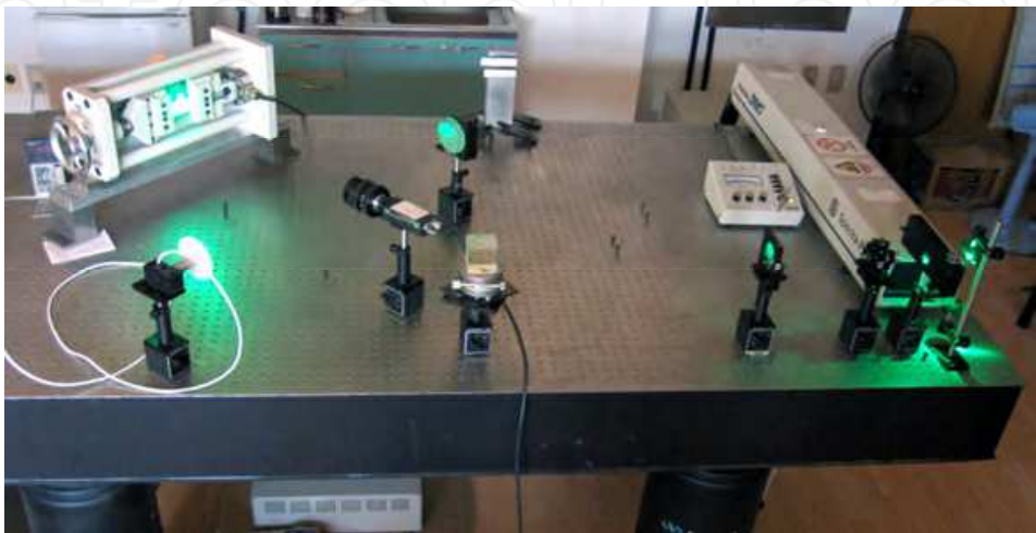
Fig. 2-3. Optical setup for measurement of in-plane displacement.
