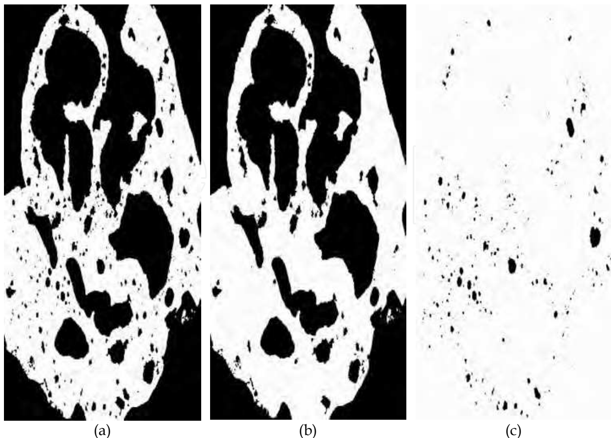
Fig. 4. Reconstructed slice showing the total porosity after binarisation (a), open porosity after region growing (b) and closed porosity (c).
