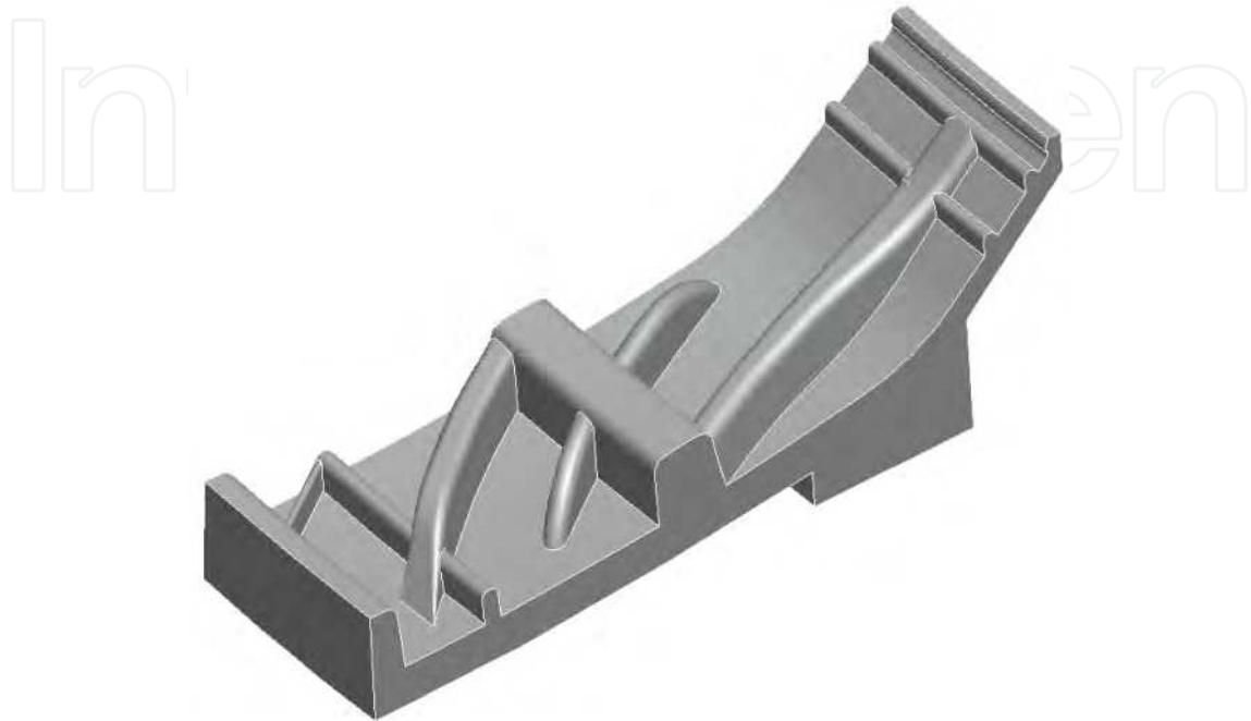
Fig. 13. Casted one-pitch-segment of tread ring.
