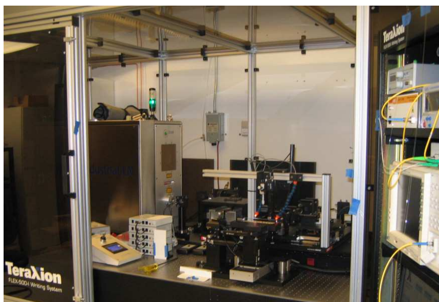
Fig. 2. Grating fabrication set up
