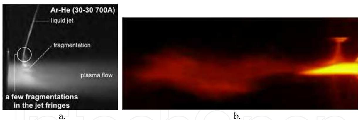
Fig. 5. (a) Example of fragmentation of an ethanol jet, about  $300 \mu\text{m}$  in diameter, starting in the fringes of a d.c. plasma jet (Ar-He: 30-30 slm, 700 A, 40 V, Anode-nozzle i.d. 6 mm) *Etchart-Salas et al (2007)*, (b) Interaction of an Ar-H<sub>2</sub> plasma jet with atomized ethanol drops *Fazilleau et al (2006)*.
