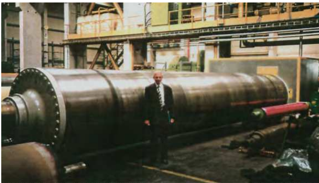
Fig. 9. Paper roll HVOF coated with WC-Co (87-13 wt %) Ducos (2006) .
