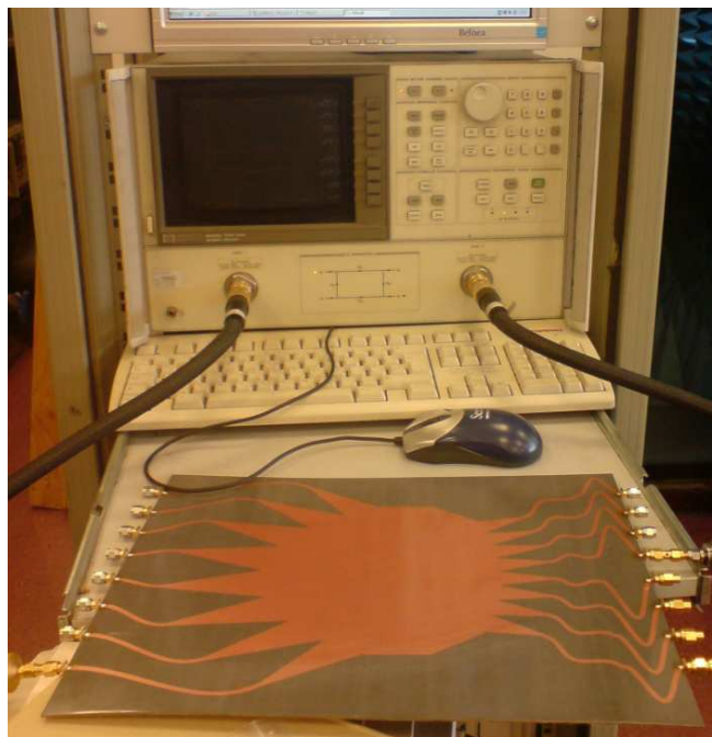
Fig. 6. Fabricated 8×8 ITS Rotman Lens Microwave BFN.
