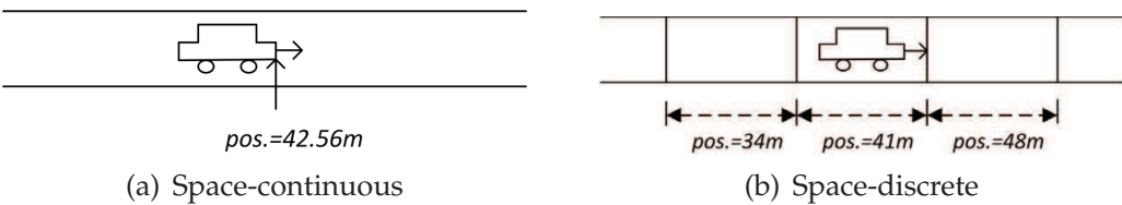
Fig. 5. The difference between space-continuous and space-discrete models.
