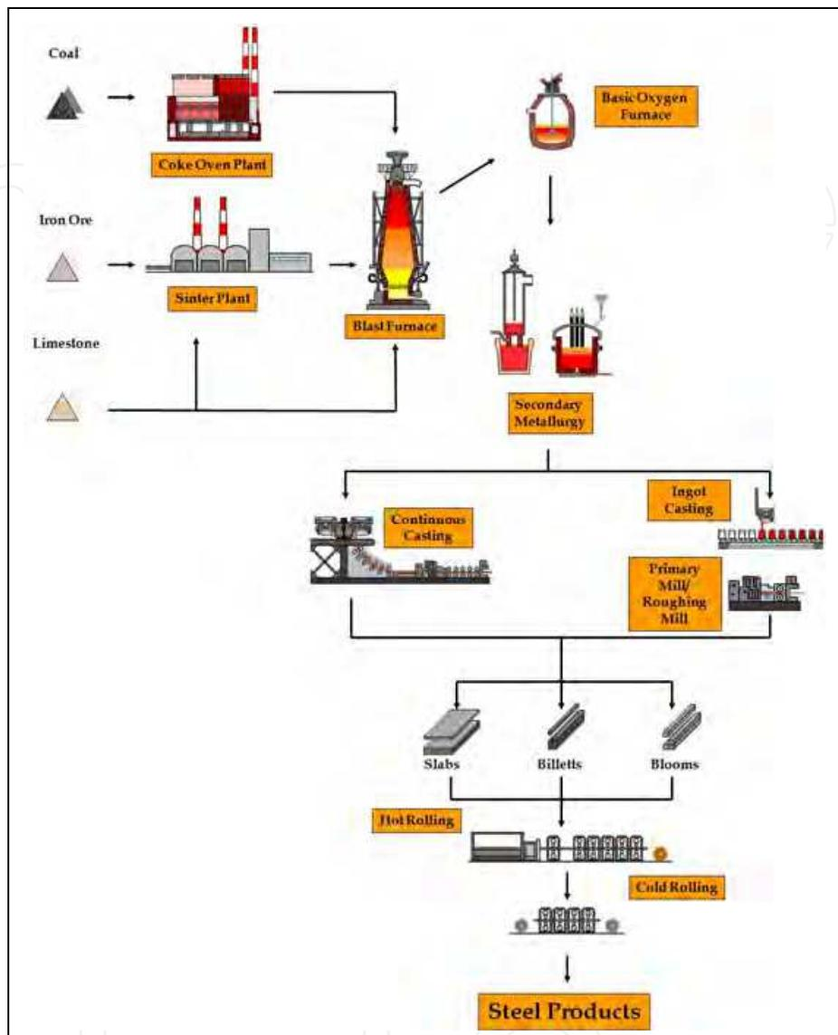
Fig. 1. The iron ore based steelmaking.
