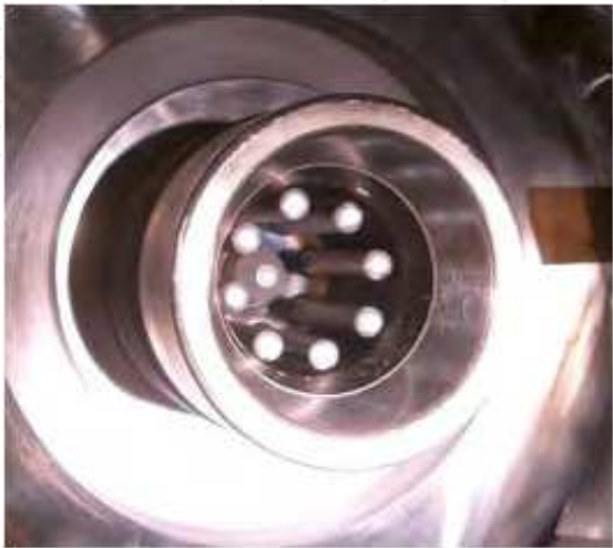
Fig. 8. Magnetoplasmadynamic(MPD) arcjet as solar wind simulator (SWS).
