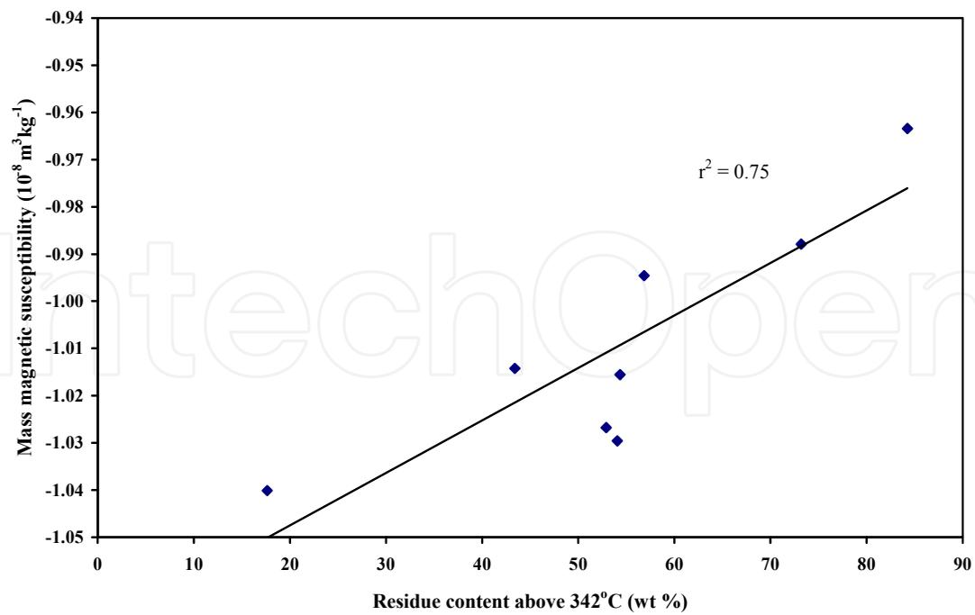
Fig. 5. Mass magnetic susceptibility versus residue content above 342 °C of crude oil samples. The measurement errors are of the order of  $\pm 0.0035 (10^{-8} \text{ m}^3 \text{ kg}^{-1})$ , close to the size of the symbols.
