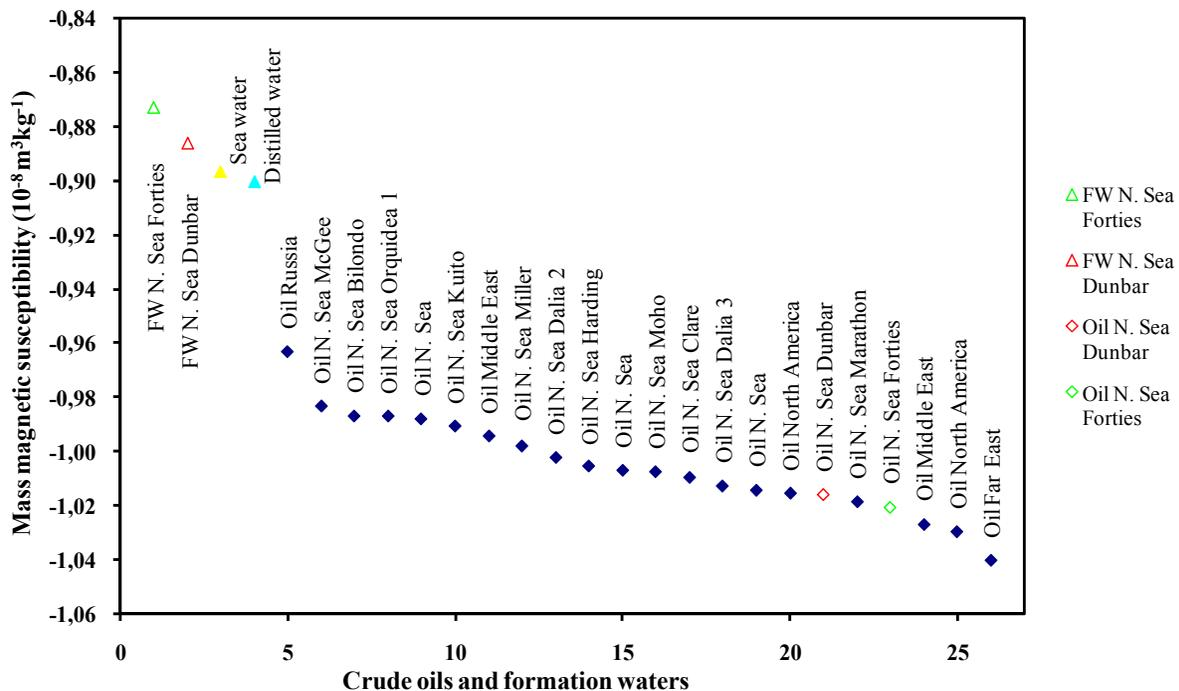
Fig. 2. Mass magnetic susceptibility of crude oils determined using a Sherwood MSB balance. The measurement errors are of the order of  $\pm 0.0035$  ( $10^{-8} \text{ m}^3 \text{ kg}^{-1}$ ), close to the size of the symbols.
