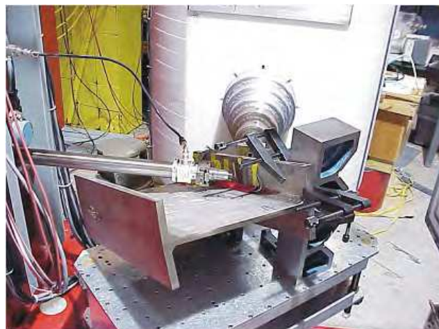
Fig. 9. Groove welded beam segment on neutron diffraction X-Y-Z translator table
