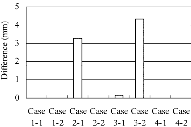
Fig. 6. Difference between the center of the blood vessel and the center of the head after deployment of the filter.
