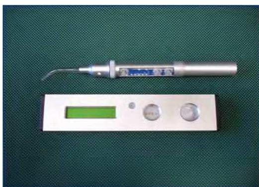
Fig. 8. Fiber-optic transillumination device (DioPower Lamp)
