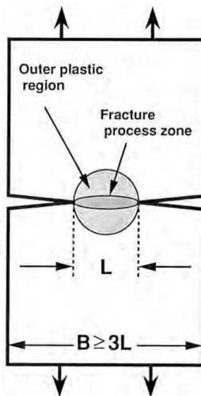
Fig. 13. Deep double-edge notched tension specimen for in-plane fracture toughness testing, showing the fracture process zone and the outer plastic deformation region (Cotterell and Reddel, 1977) ( $B$ : specimen width,  $L$ : ligament length).
