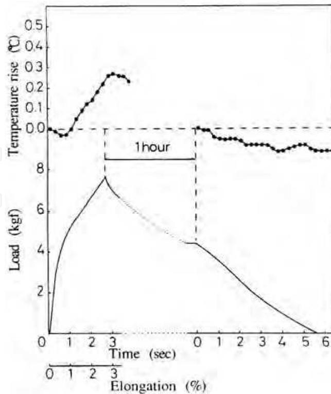
Fig. 7. Changes of load and temperature of paper during tensile straining, stress relaxation, and destaining periods (Yamauchi and Tanaka, 1994).
