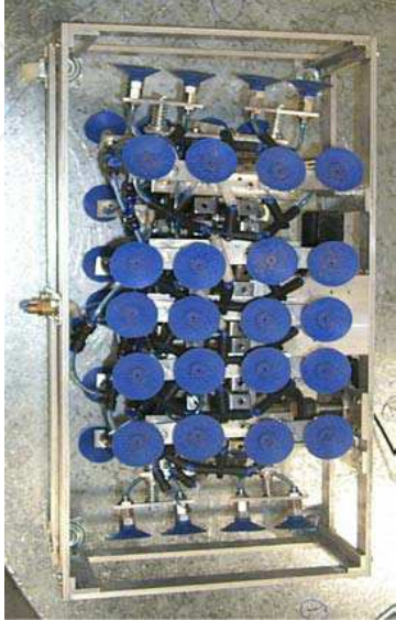
Figure 2.3 Climbing robot Cleanbot III
