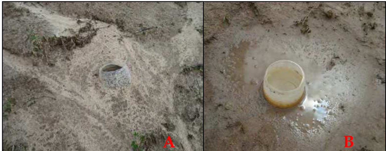
Fig. 3. Presence of water in the physical protector (A) and burial through laminar erosion (B) after rainy season in a pasture area located in the municipality of São Cristovão, Sergipe, Brazil, after the implementation of direct sowing (Source: Santos, 2010).
