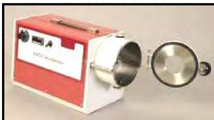
Fig. 8. Accelerator abrasion tester
