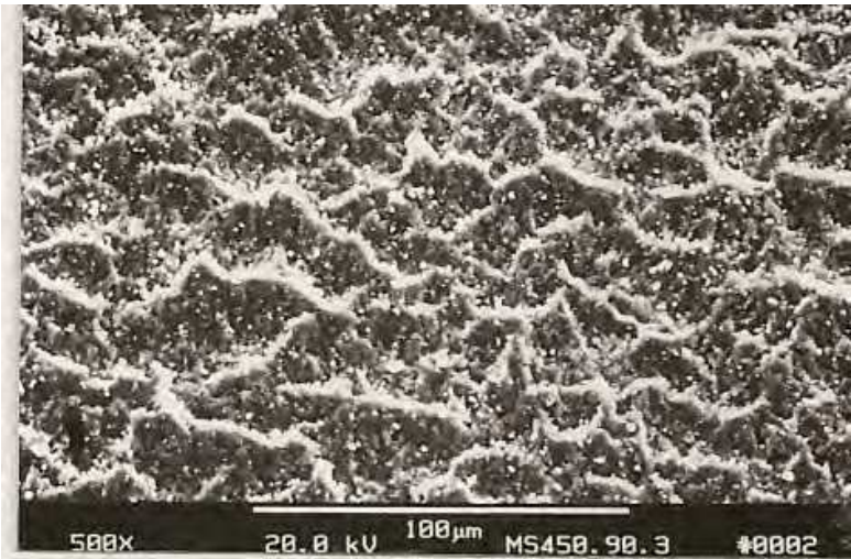
Fig. 8. Scanning electron micrograph of mild steel exposed in the FB rig at 450°C and 2.5 m s -1 .
