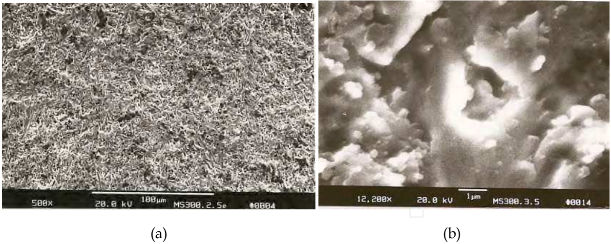
Fig. 7. Scanning electron micrograph of mild steel exposed in the FB rig at 300°C and 2.5 m s -1 showing a) the surface morphology and b) morphology at higher magnification
