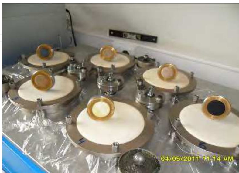
Fig. 6. Martindale abrasion tester prepared for wet abrasion
