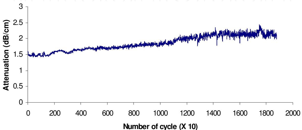
Fig. 16. Variation of ultrasonic attenuation with fatigue life
