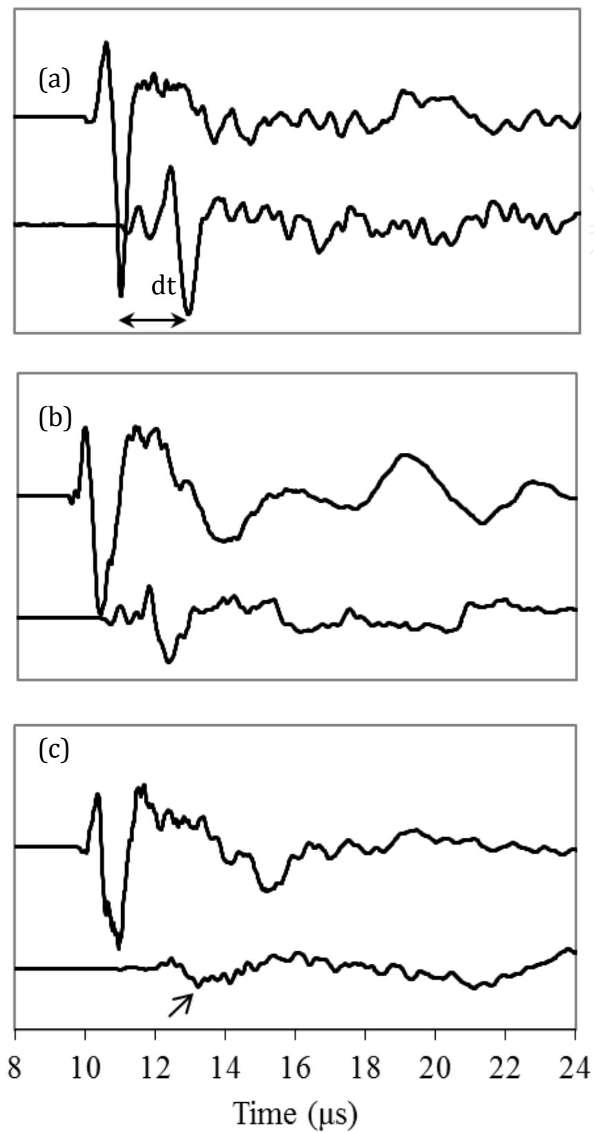
Fig. 2. Sample waveforms of 1<sup>st</sup> and 3<sup>rd</sup> receiver for mortar with inclusions contents 0% (a), 1% (b) and 10% (c) and inclusion size 30x30x0.5 mm.
