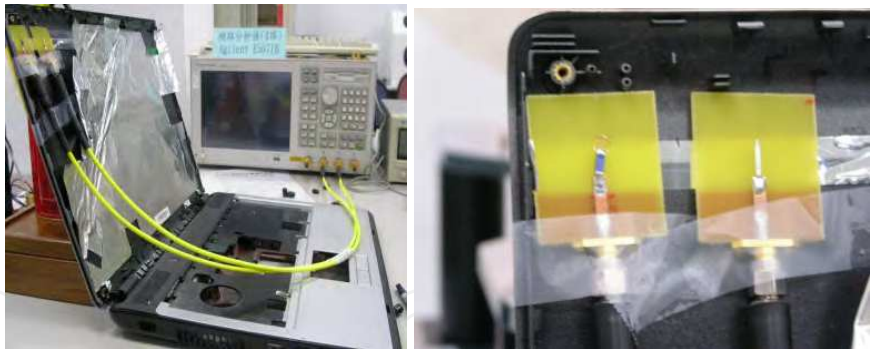
Fig. 36. Placement of two chip antennas inside mold.
