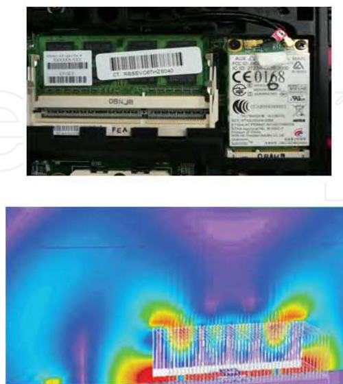
Fig. 47. RF module location and nearby field distribution.
