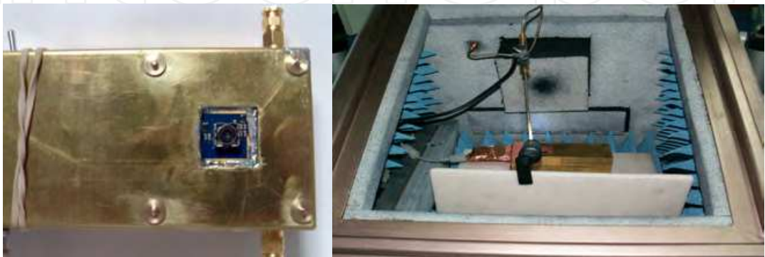
Fig. 46. Shielded enclosure and loop probe for noise measurement of camera module.
