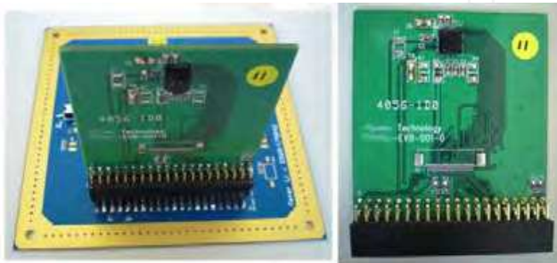
Fig. 56. Physical camera connected to testing board.
