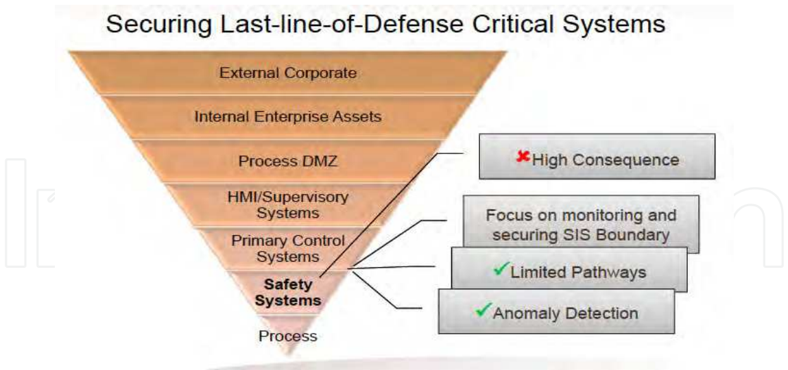
Fig. 19. Position and mechanisms enabling Last-line-of-Defense.
