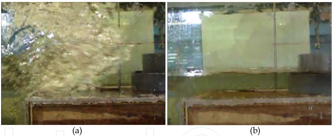
Fig. 19. Snapshots of inundation wave against weir Type B 2 with: (a) h_1=0.03\text{m} caused large weir overtopping and (b) h_1=0.02\text{m} caused small weir overtopping
