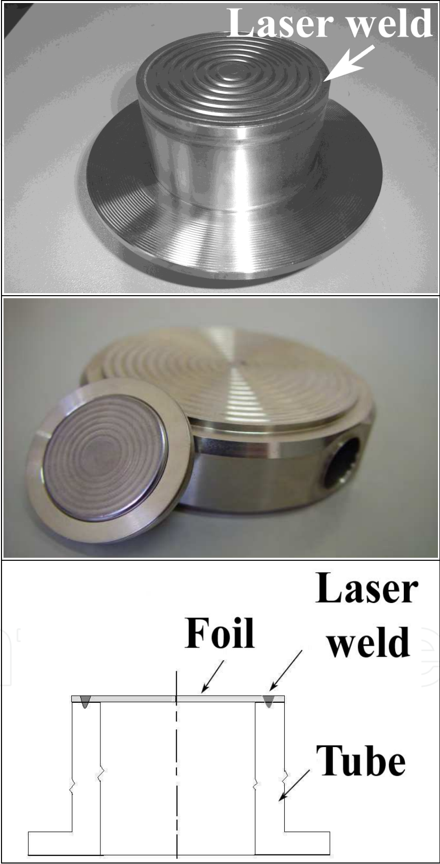
Fig. 1. Chemical seal welded by pulsed Nd:YAG laser.
