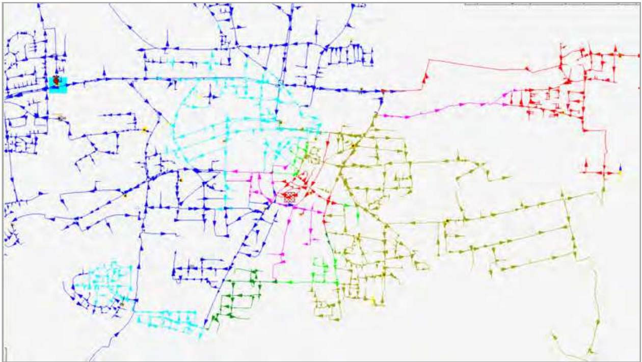
Fig. 8. Detailed view of calorific value distribution in the inner city area network (distinction by color)
