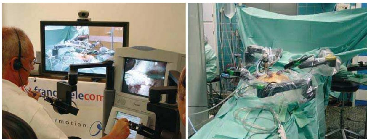
Fig. 2. The Zeus robot during the first intercontinental surgery, the colecystectomy was performed on the patient in Strasbourg from New York. (Photo: IRCAD)
